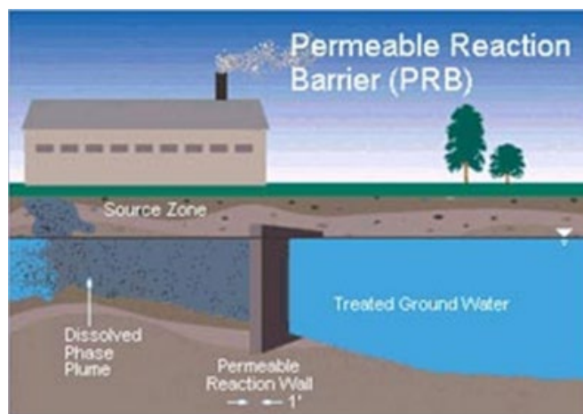
Figure 11. Schematic of Permeable Reactive Barriers (PRBs).
